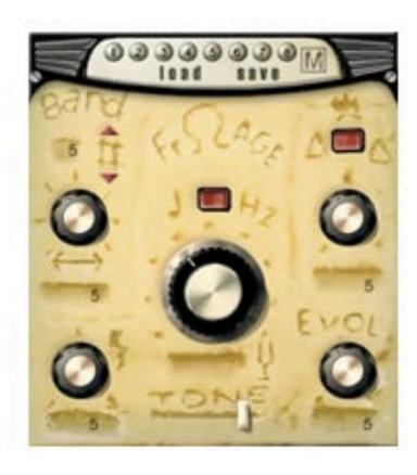
Frohmage is a multi-band resonant filter. It can offer some unique sounds, from slow and deep filter sweeps to the most savage tones with high resonance setting and heavy distortion.
